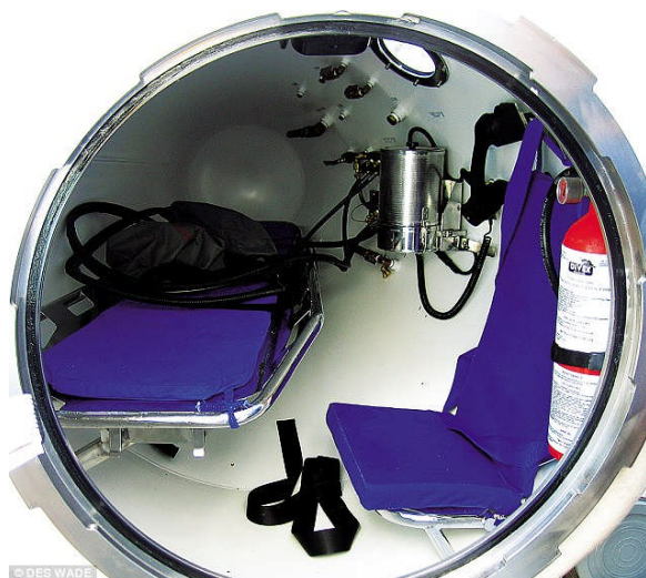
Inside the portable chamber, in which a patient and an attendant can be airlifted to hospital while under pressure
