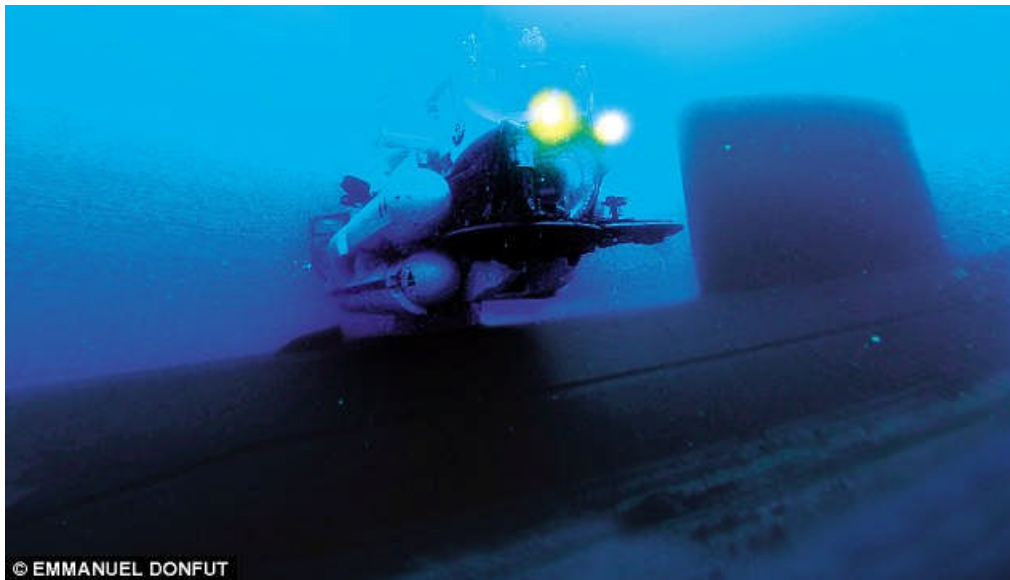
The Nato submarine rescue vehicle (SRV) mates with a bottomed sub. Nemo is the most advanced in the world and is jointly owned by Britain, France and Norway.
